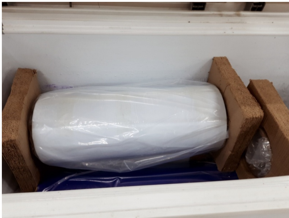
Prepreg storage in deep freezer
